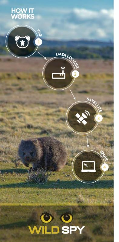
wild Spy WIDs are animal-borne transmitters with a configurable range of 20-200m line of sight. Each WID transmits a unique identifier which is picked up by a data logger when in range. WID data loggers record tag ID, time and duration of log, and received signal strength (RSSI). WIDs come standard in the form of an ear tag or can be designed in virtually any format (including collars) to suit most species, including small mammals, birds and reptiles.
